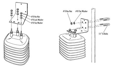
Attaching Solar Radiation Shield to Mounting Bracket
