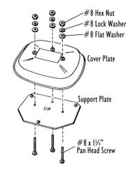
Attaching Support Plate to Cover Plate
