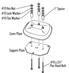
Attaching Support Plate to Cover Plate
