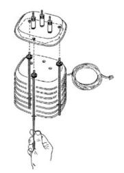
Attaching the Cover Plate Assembly to Solar Radiation Shield
