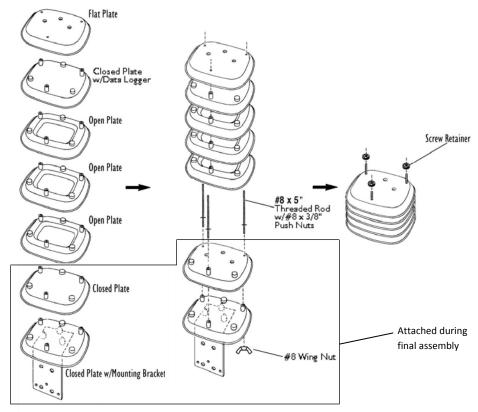
Assembling the Radiation Shield Plates
