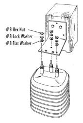
Attaching Solar Radiation Shield to Mounting Bracket
