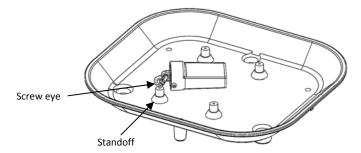
To attach a HOBO Water Temp Pro v2 (U22-001) or a HOBO Pro v2 Internal Temp/RH logger (U23-00x) to the Solar Radiation Shield, place the logger in the clamp provided in the U23 Clamp Kit. Secure the clamp into the standoff on the closed plate as shown with the screw and washer provided in the kit. Note: The HOBO Water Temp Pro v2 can be mounted into the shield using the U23 Clamp Kit, but the clamp fit will not be as snug as it is for the HOBO Pro v2 Internal Temp/RH logger.
