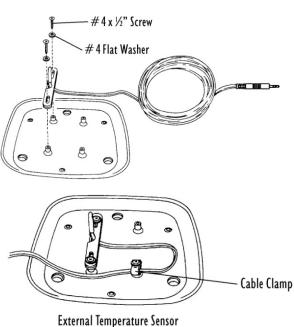
bulge side down. Tighten the screw completely so that the cable cannot move within the cable clamp.
