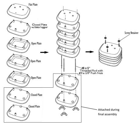
Assembling the Radiation Shield Plates
