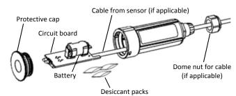
4. If the logger has an O-ring around the battery clips as shown in the photo in step 7, remove and discard it.
