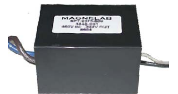
Magnelab AC Potential Transformer
